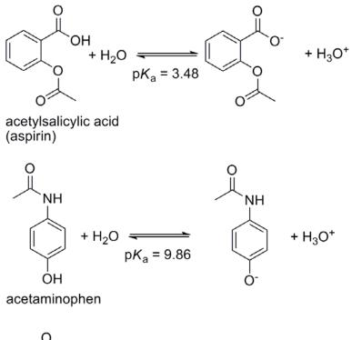
Aspirin and acetaminophen are both weak acids, but they have very different  $pK_as$  that allow them to be separated from each other by using aqueous extraction solutions of different pH (< 10 to remove aspirin, > 10 to remove acetaminophen.
