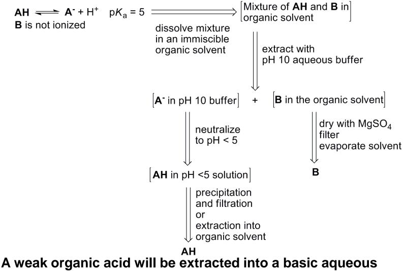
buffer as its conjugate base, a weak organic base would be extracted into an acidic aqueous buffer as its conjugate acid.
