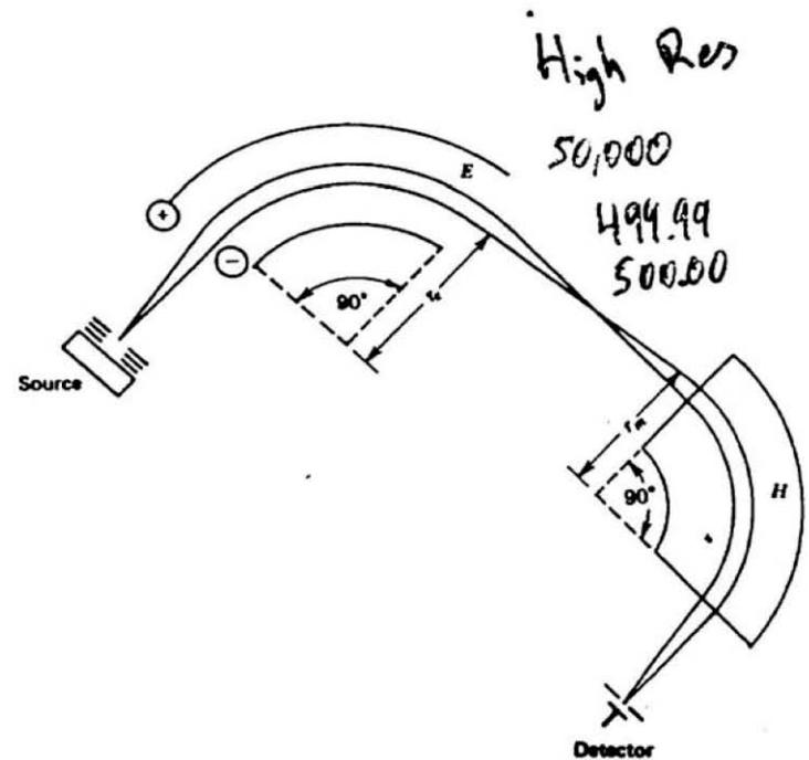
Figure 4. Nier-Johnson double-focusing mass analyzer. E = electric field, H = magnetic field.
